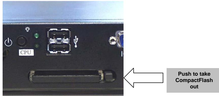
Figure 7: CompactFlash Adapter
