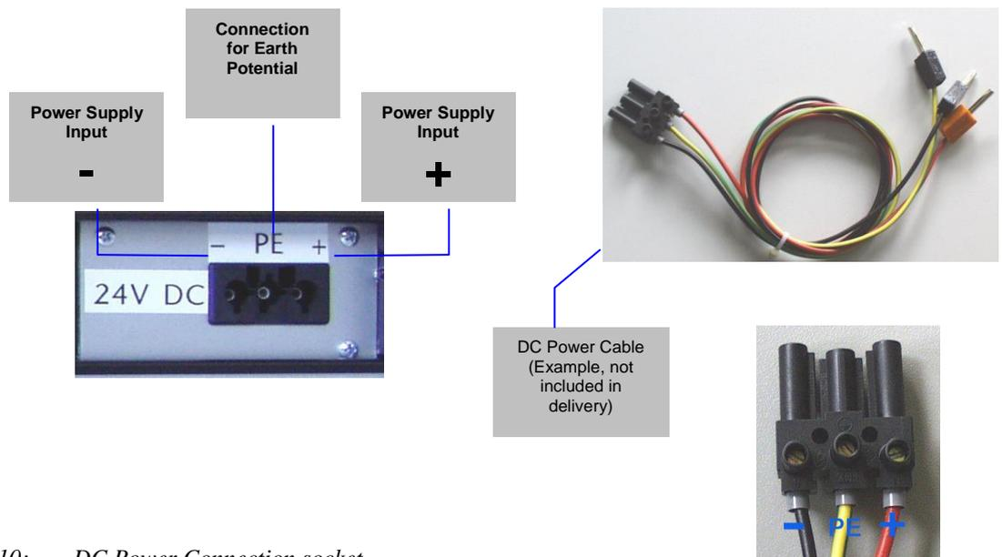
Figure 10: DC Power Connection socket
