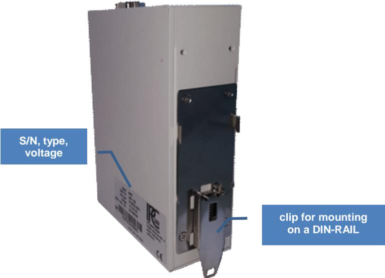
Figure 2: MEC2 rear view
