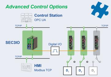
To meet higher demands on the monitoring and control options of the *ERM1*, the integration of **ip4Cloud/SEC3IO** offers numerous additional functionalities. On the one hand, it enables the automation of the *ERM1* network selector using standardized communication protocols (e.g. SNMP, REST, OPC UA, MQTT). On the other hand, the status of an *ERM1* 1-port Ethernet A/B switch can be monitored and controlled via its integrated web interface.
