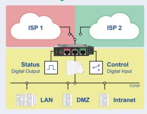
With *ERM1*, you can easily toggle between two Internet service providers (ISPs) to maintain smooth access to telecommunication lines even in the event of disruptions and outages of one provider.
