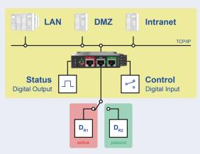
Redundant systems are commonly deployed to ensure the operation and reliability of critical systems. Yet many devices do not meet this requirement. With *ERM1* even these devices can be used for redundant operation.
